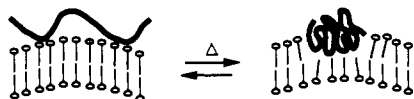
Figure 2. Schematic illustration of the interaction of NIPAM-C18 copolymer ( 2 ) and NIPAM homopolymer ( 3 ) with liposomal membranes below (no influence on lipid flip-flop) and above (enhanced lipid flip-flop) the polymer's LCST (cloud point temperature).
